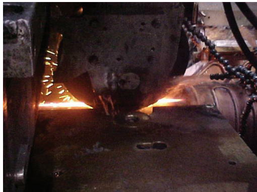
Figure 3: The tube leaving the high-frequency induction coil and passing through the weld pressure rolls
