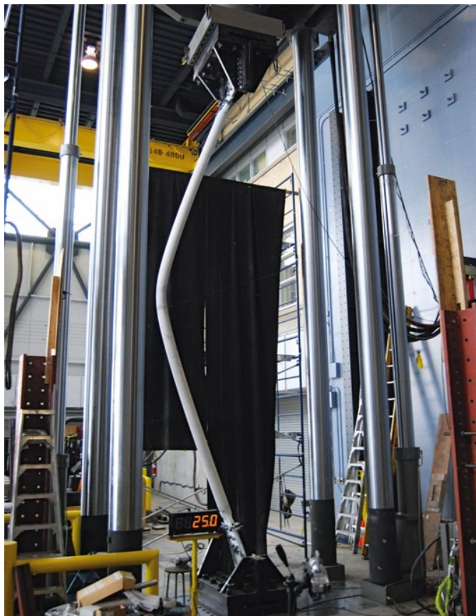
Fig. 5. Cold-formed CHS brace during the compression cycle of a seismic loading protocol, in a 12 MN-capacity universal testing machine
