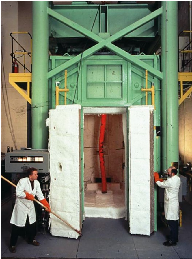
Fig. 3. CFSHS in a column-testing furnace
