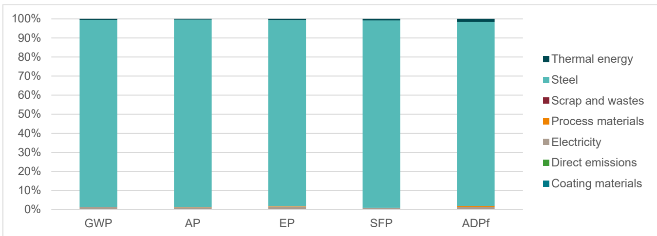
Figure 2: Relative contribution by manufacturing component for 1 metric ton of hollow structural sections
