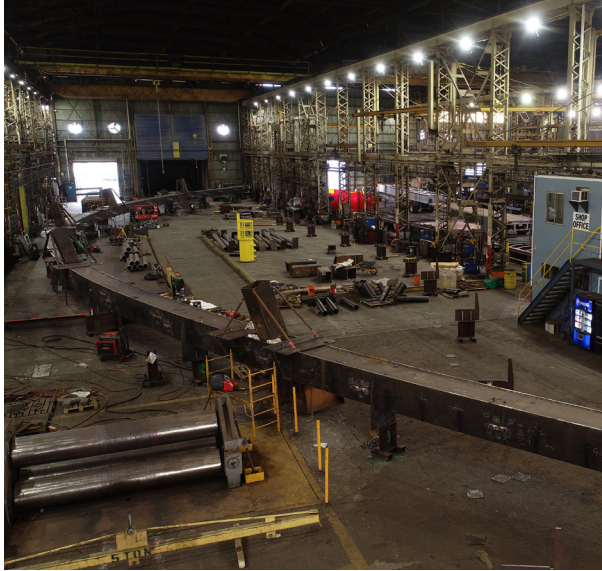
HSS22x22x7/8 stubs being set for attachment to the built-up arch ribs. The inclined ribs made for complex geometry with tight tolerances.
