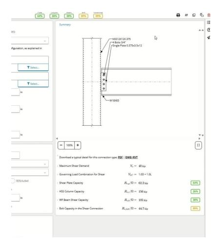
For example, if we were to navigate to the **Bolt Inputs** section and change the number of bolts to 5 instead of 4, the graphic would respond accordingly.
