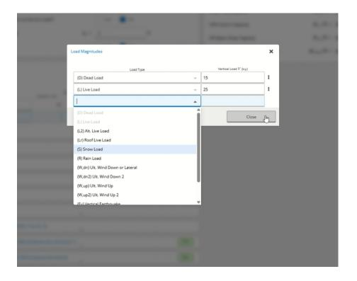
Below the **Load Magnitudes** section, there are more sections with other load parameters such as basic geometric properties of the column and beam to edge distances can be adjusted. Even further down in the calculator, there are more sections that can be expanded to see the equations going into the connection.
