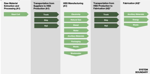
All A1 steps represent manufacturing of unfabricated HSS by Atlas Tube. Stages with an asterisk rely on data from the AISC & STI industry average EPD for fabricated HSS (AISC & STI, 2022). This EPD does not declare the modes of transportation used in A2, so it is assumed all common modes (truck, ship, rail) are used.
