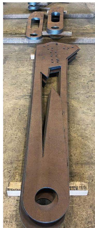
A gusset plate sporting the MrBeast logo. Circular holes in the foreground accept 6" solid pins used to anchor the tension rods, end and center sections.
